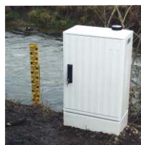
protection housing with puck antenna, modem inside
